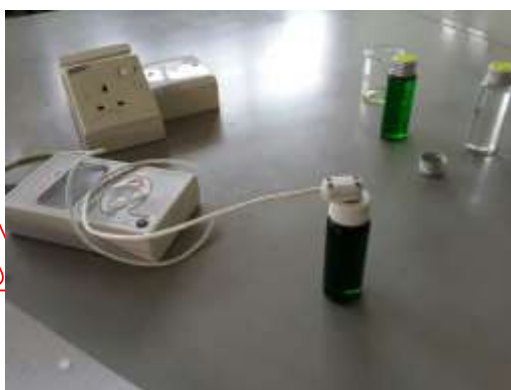
Figure 3.8: Thermal conductivity test of ethylene glycol at room temperature
