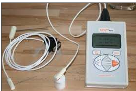
Figure 3.6: KD2-Pro Thermal Properties Analyzer
