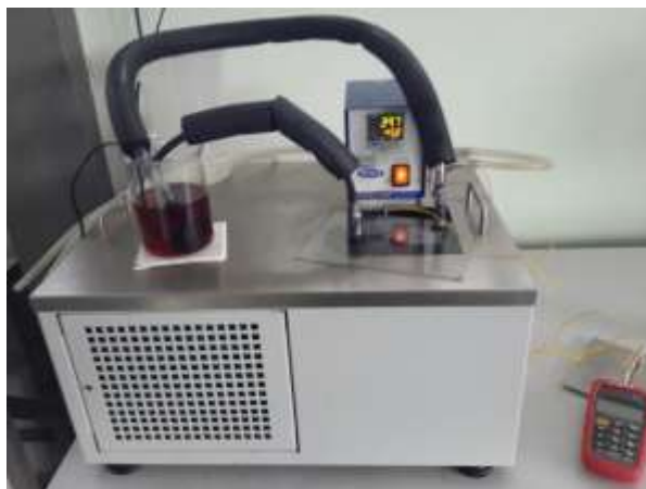
Figure 3.10: Set up of heat transfer coefficient test
