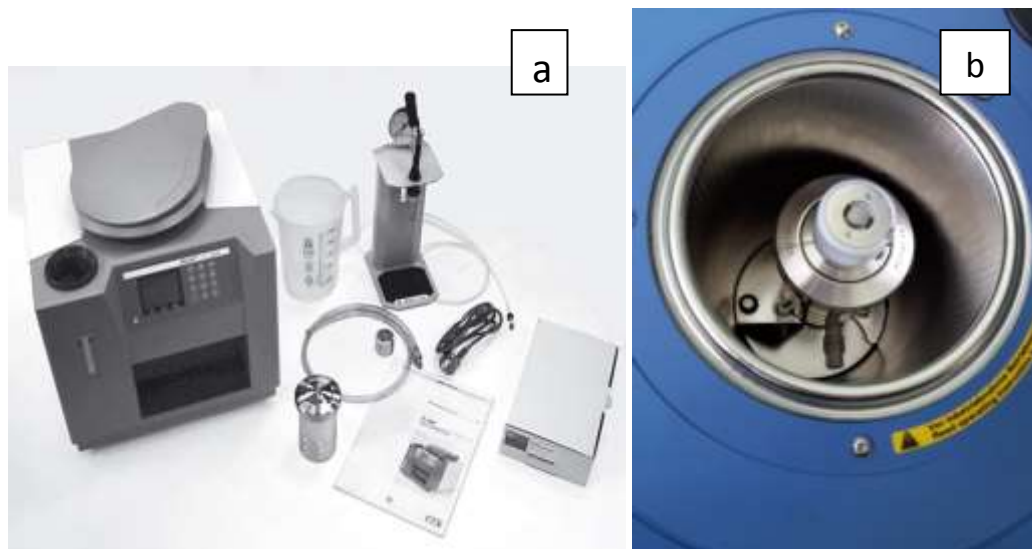
Figure 3.9: (a) Complete set of Calorimeter Bomb, (b) Position of decomposition vessel inside the vessel of calorimeter.
