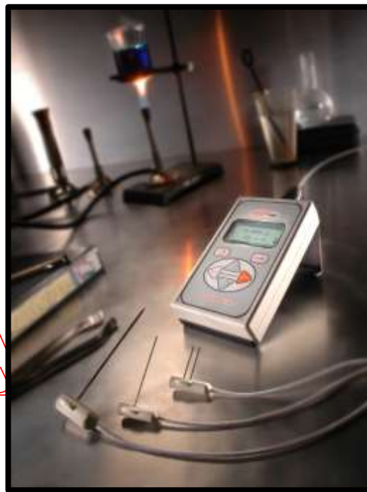
Figure 3.3: KD2 Pro Thermal Properties Analyzer
